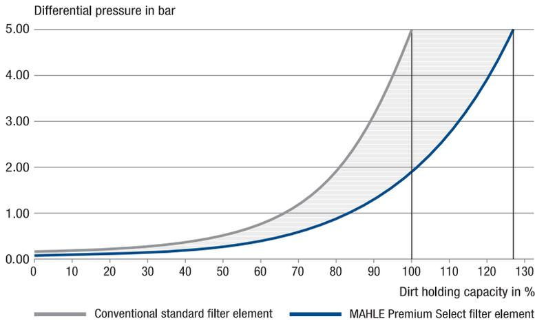
*Continuously higher performance plus longer service life: innovative MAHLE Premium Select filter element with 30% more dirt holding capacity, lower differential pressure, and an optimized differential pressure profile—for reduced energy consumption.*
